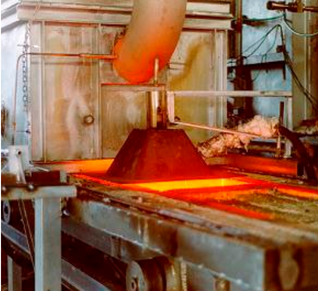
Laboratory furnace for direct reduction test
